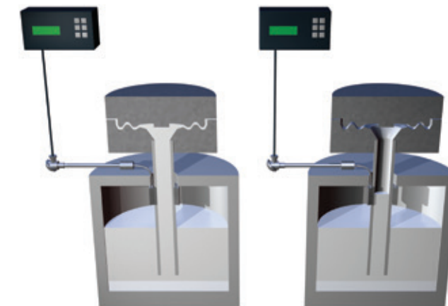
RP used to control the metal level in a riser tube.
